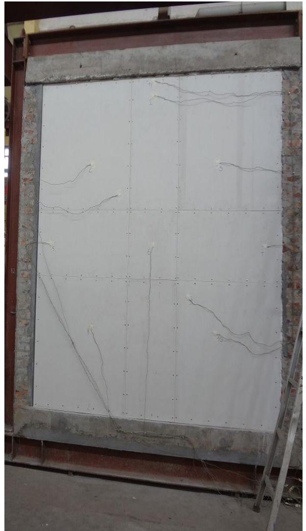
Independent fire testing at nearly 2000 degrees (F) for more than two hours to meet Singapore fire standards, the most stringent in the world
